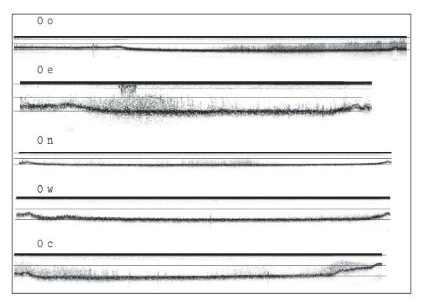
Figure 4.2: Acoustic traces of transect lines in Lake Omapere. For location of transects see Figure 4. Length of each transect were as follows: Oo – 3.68 km (West to East), On – 1.19 km (South to North), Ow – 3.61 km (East to West), Oc – 2.89 km (North to South) and Oe – 2.58 km (South to North). Macrophytes appear as lines above the lake bottom where their density exceeded 5%. Horizontal lines in each transect represent 1 m depth intervals.
