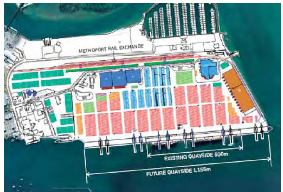
Figure 61. Planned extension of container berth at POT
