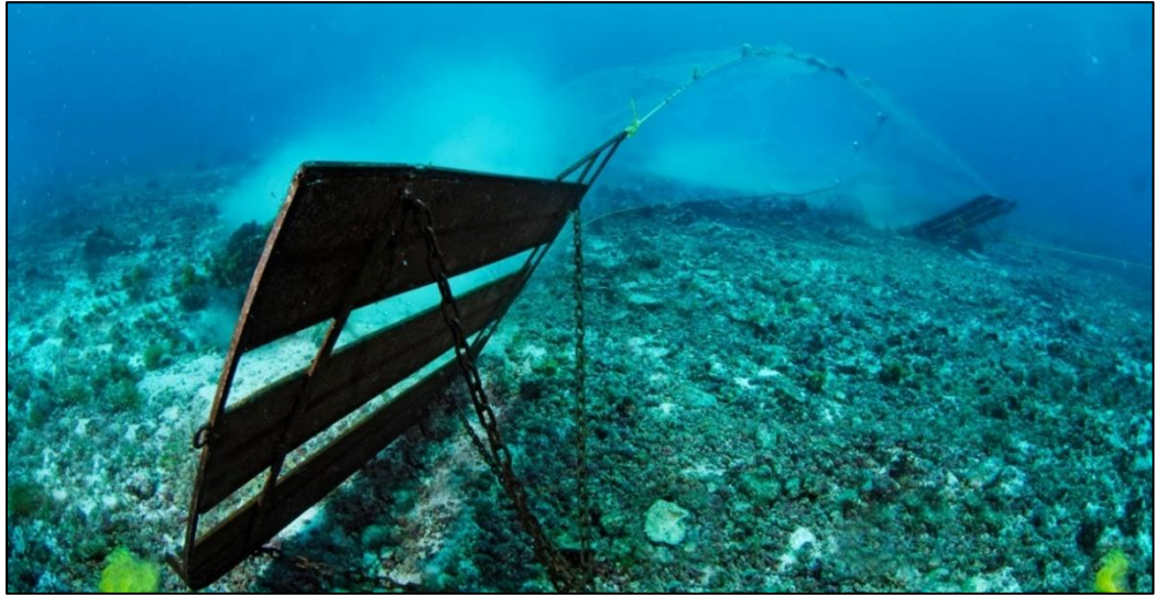
Figure 6 Trawl door (otter board) and net 19
