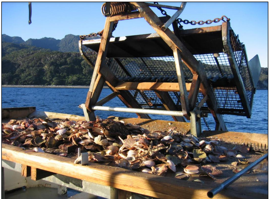
Figure 7 Example of a box dredge typical of those used in the Northland SCA 1 and Coromandel SCA CS commercial scallop fisheries in northeastern NZ
