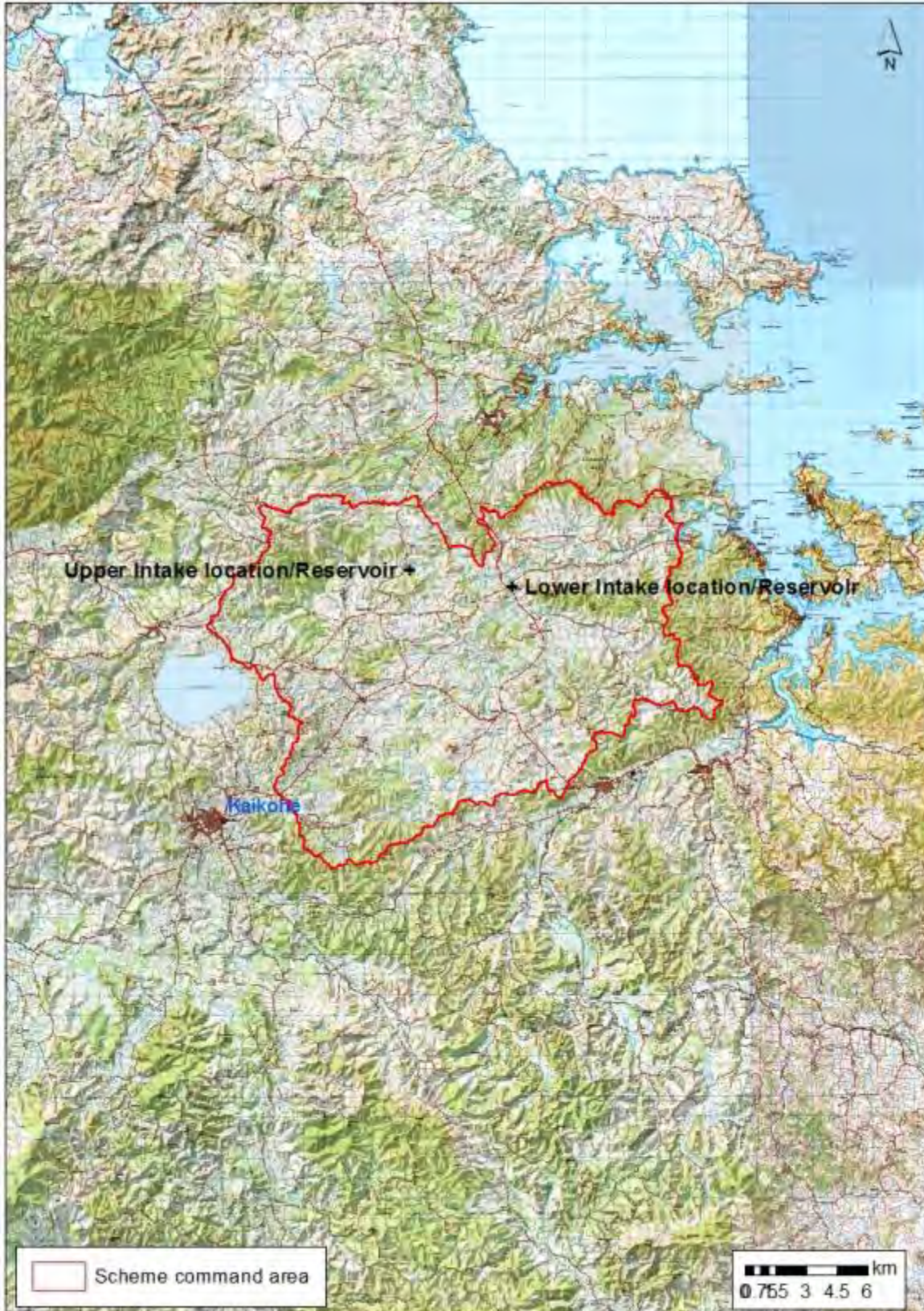
Figure H.9 – Approximate locations of intakes for water harvesting or instream dams for the Waimate North Area
